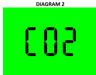
When DIP Switch 2 is ON the LCD will simply display 'CO2'
